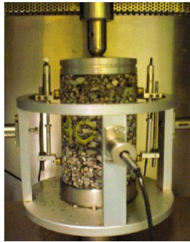
Dynamic Modulus Test
