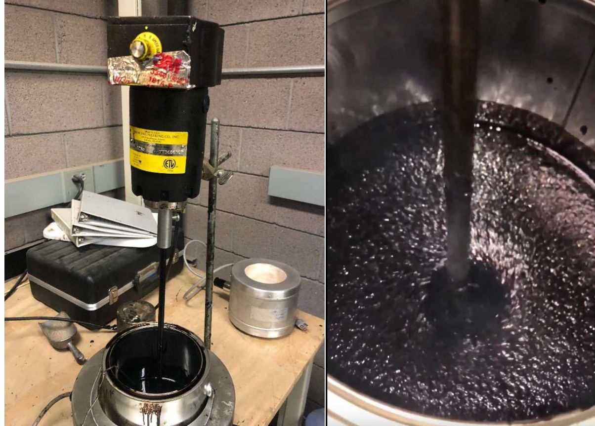
Blender and closeup view of CRMB binder preparation
