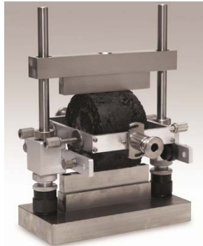
Resilient Modulus Test
